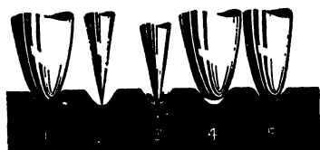
Phonograph needles. 1, theoretically ideal but impractical because needle angle changes; 2, too sharp, allowing free movement; 3, too sharp, causing gouging; 4, too blunt, scoring groove walls; 5, best practical shape.
